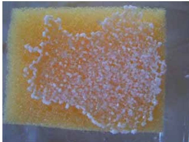
Fig 15 Salt crystals reformed after being dissolved by rain water in a couple of days. (Most did not soak into this fine sponge - a coarser sponge was needed to show infiltration better.)
